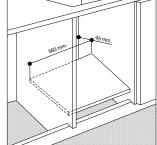
The panels of the adjacent cabinets must be made of heat-resistant material. In particular, cabinets with a veneer exterior must be assembled with glues which can withstand temperatures of up to 100℃.
