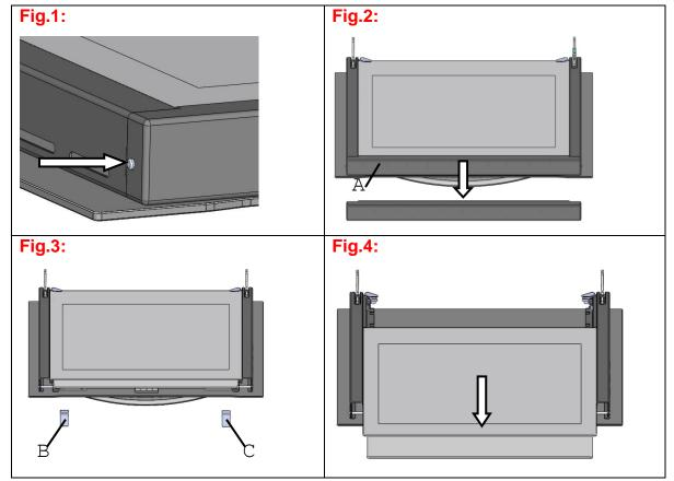
Method 2 remove and assemble procedure:
