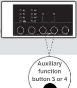
You may make the programme active by pressing the pre-wash button on the display panel when the led light of the  $\sqcup$  symbol turns on.
