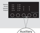
You may make the programme active by pressing the rapid wash button on the display panel when the led light of the [>>) symbol turns on.
