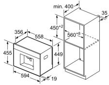
Bean and water containers are removed from the front. Recommended installation height 95-145 cm. me measurements in mm
